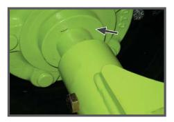
**Metal Axles Seal Guards** protection over hubs, with bolt in replaceable axle
