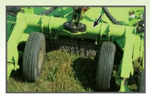
**Rear Beam** The centre section wheel standard uses a large 6" O.D. x 5.5" I.D tube. The lifting system is symmetrical, resulting in an even loading on both sides of the centre frame. Spring steel bushings and high carbon steel pins are used at all major pivot points.
