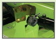
Wing Lift lock up with rubber stopper
