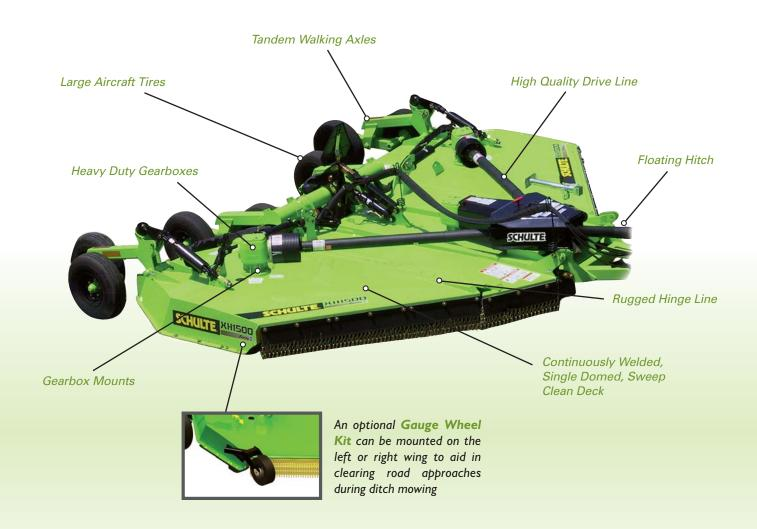
**Drive Line** A four gearbox drive line arrangement with a forward mounted power divider allows the use of individual slip clutches to protect the cutter. The four gearbox drive line allows the wings to operate at angles from  $25^{\circ}$  down up to transport position.
