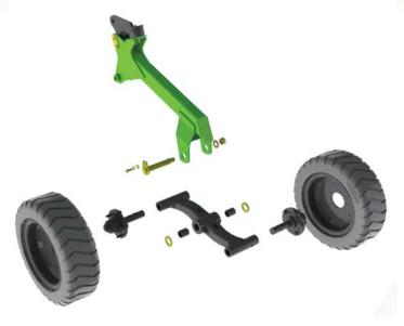
**Swivel Hitch** A swivel hitch allows the cutter to move over rough terrain without the hitch clevis binding up onto the tractor drawbar. The swivel assembly uses a strong 2" main shaft. Should the assembly loosen up over time machine bushings can be added to maintain a snug fit. A spring steel bushing protects the hitch frame from wear.
